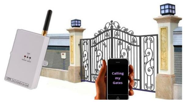
GSM door opener is a GSM switch remote control system which can activate automatic gates with a free call from you mobile phone. The users' phone numbers are programmed into the device by SMS. The device recognizes incoming Caller ID and drop the call before switching. With this system you can authorize up to 99 mobile phones to open the gate at no cost. This system has two models N/O,N/C output
